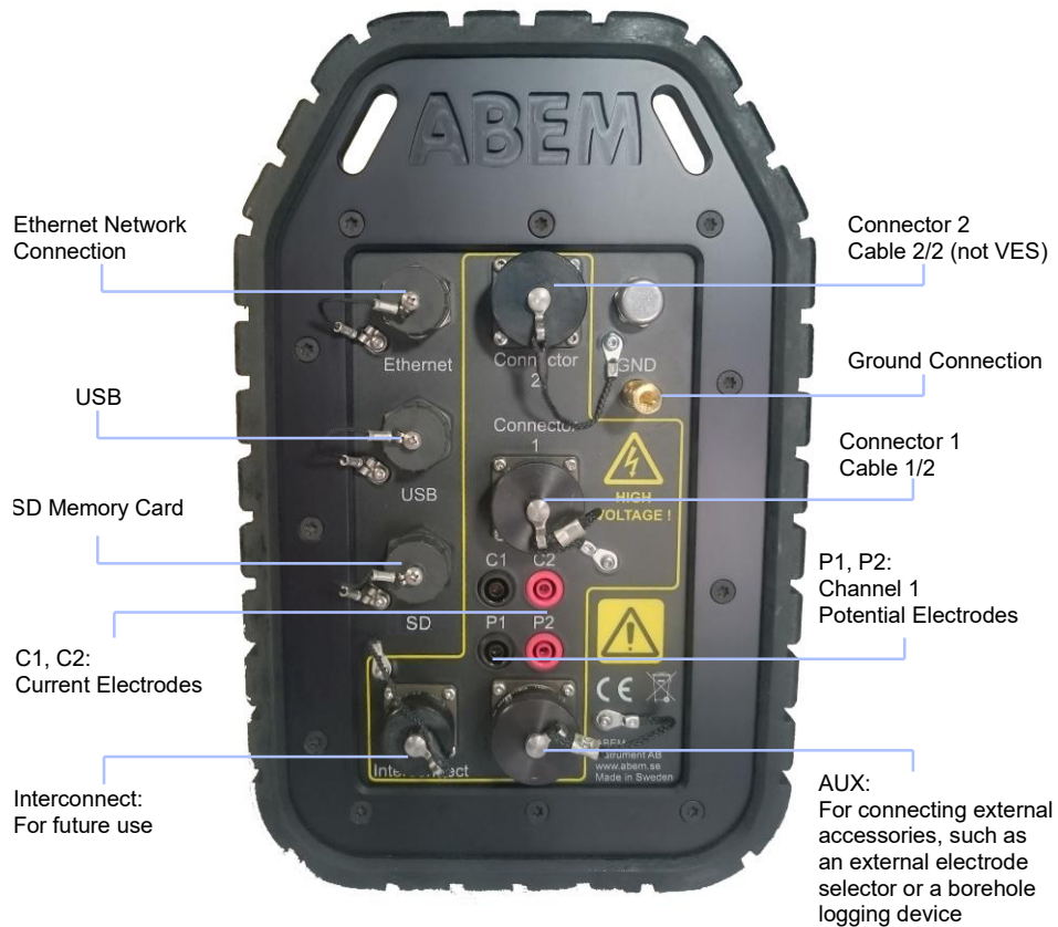
Figure 3 The connector panel of the Terrameter LS 2
