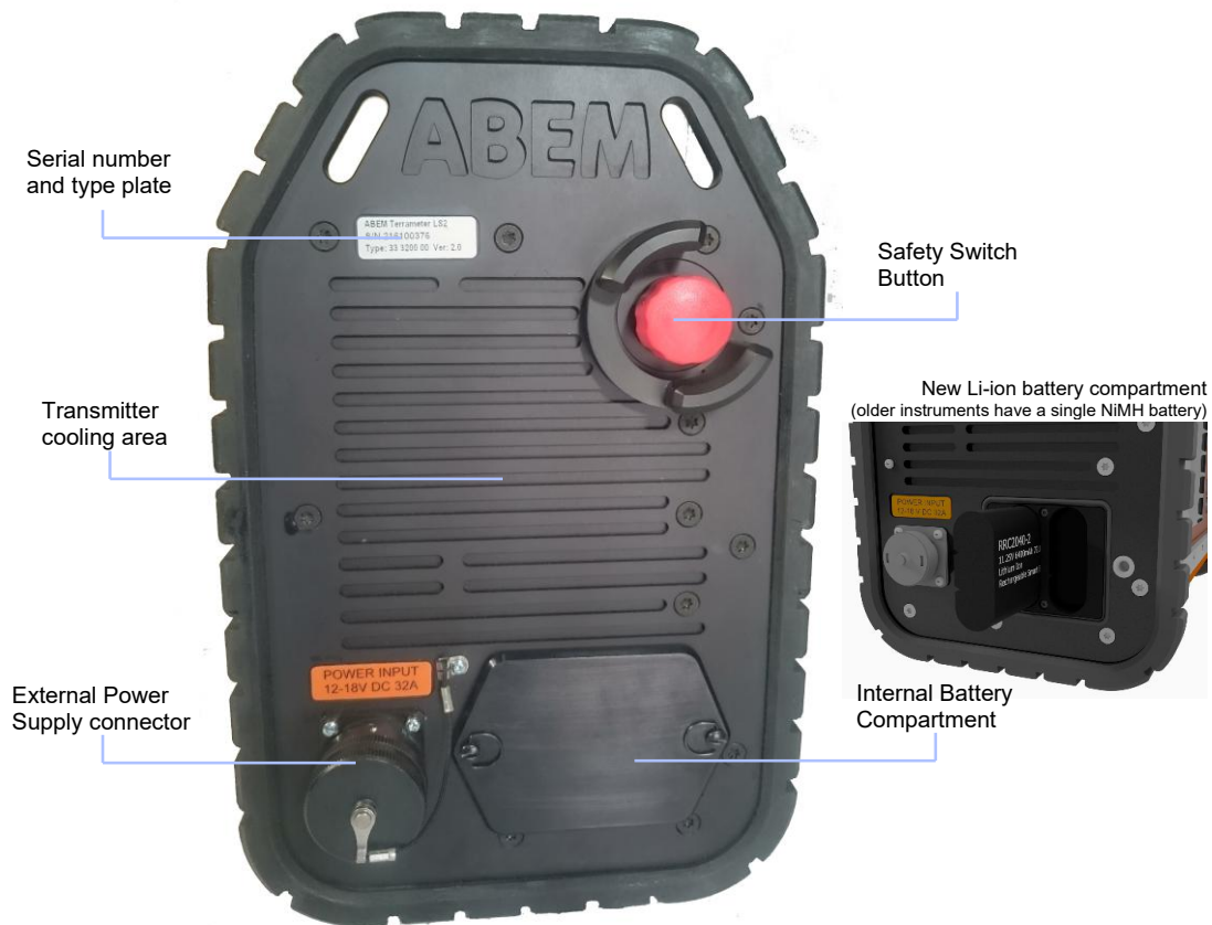
Figure 4 The power panel of Terrameter LS 2
