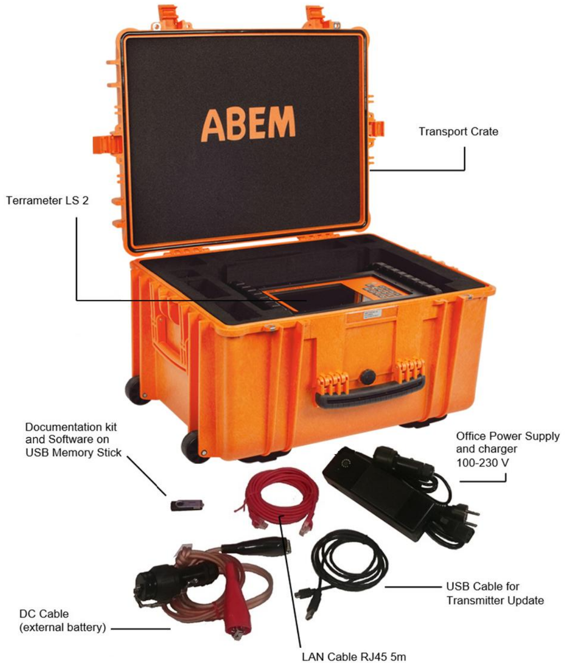
Figure 2 The Terrameter LS 2 instrument package
