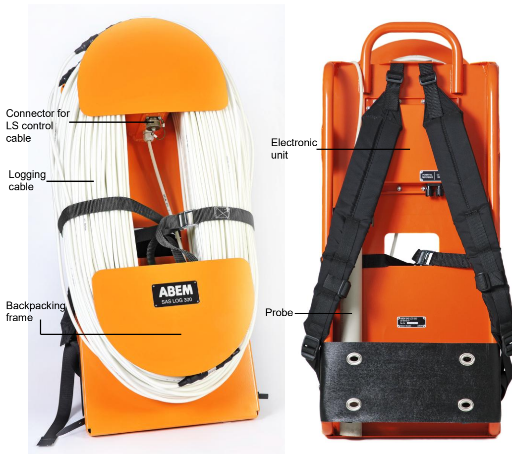
Figure 81 Terrameter Log 300 with backpacking frame
