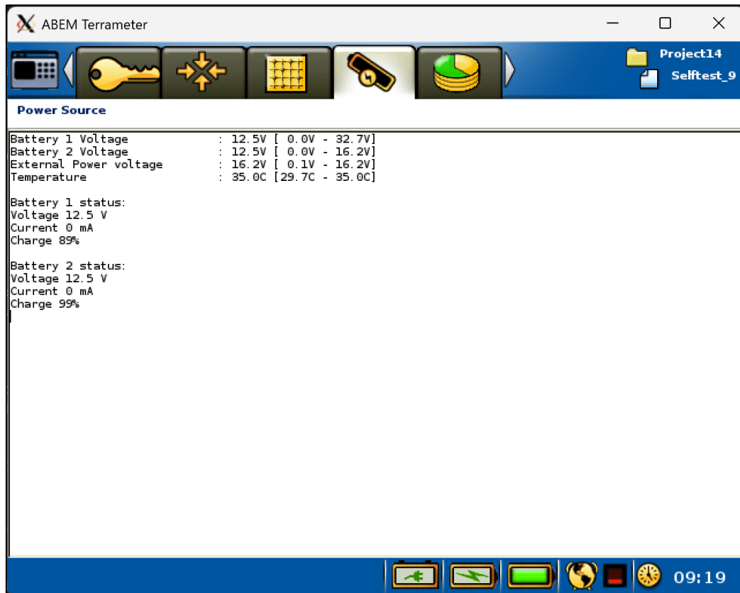
Figure 40 Status Page for power supply and temperature
