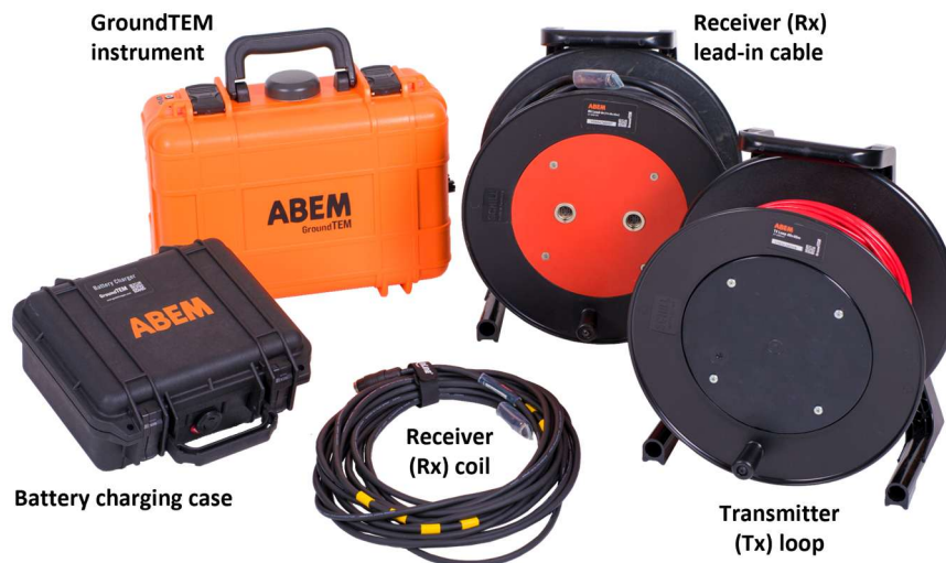
Figure 3. Main components of the GroundTEM system (apart from the shipping case and two Li-ion batteries).
