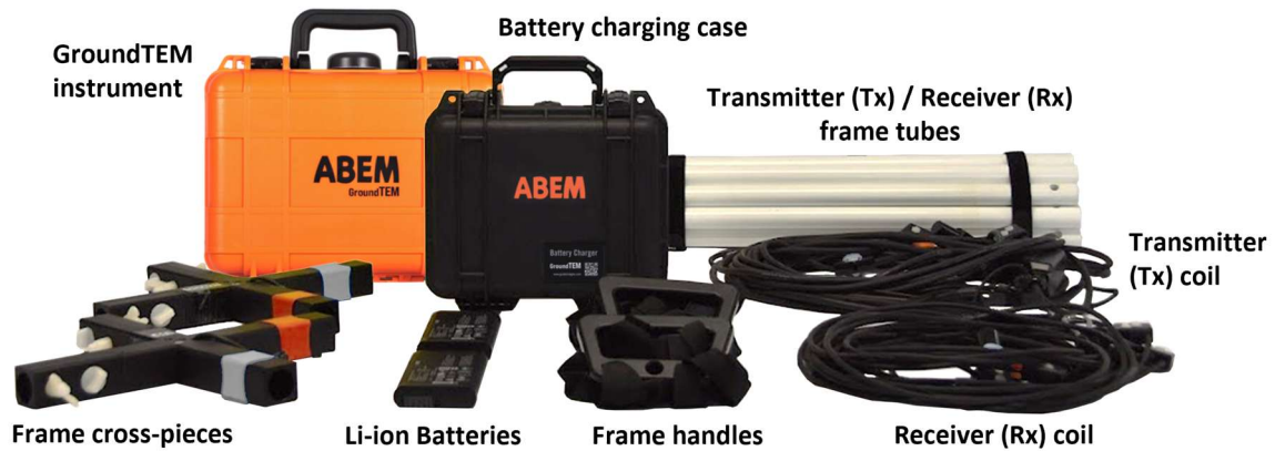
Figure 10. Main components of the GroundTEM system with Explorer Coils, the total system weight for a GroundTEM setup including GroundTEM unit and Explorer Coils is approximately 19.5 kg (excl. battery charging suitcase).
