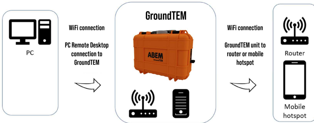
Figure 23. Flowchart for how to put GroundTEM unit online.
