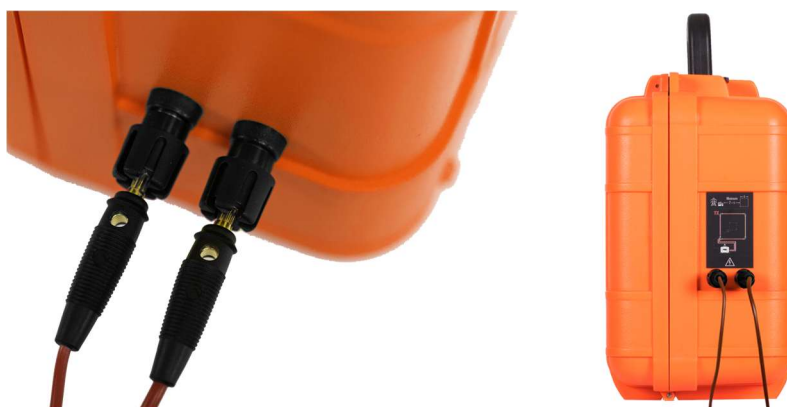
Figure 7. GroundTEM banana plugs. Connect Tx loop in any order.
