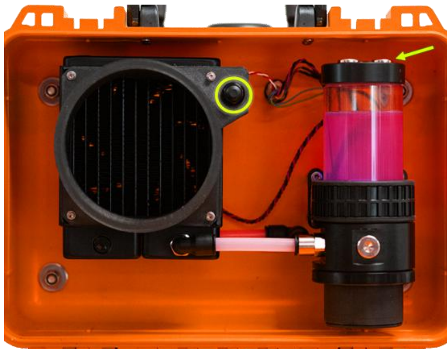
Figure 4: Coolant compartment of TX unit with bypass button indicated in red circle.
