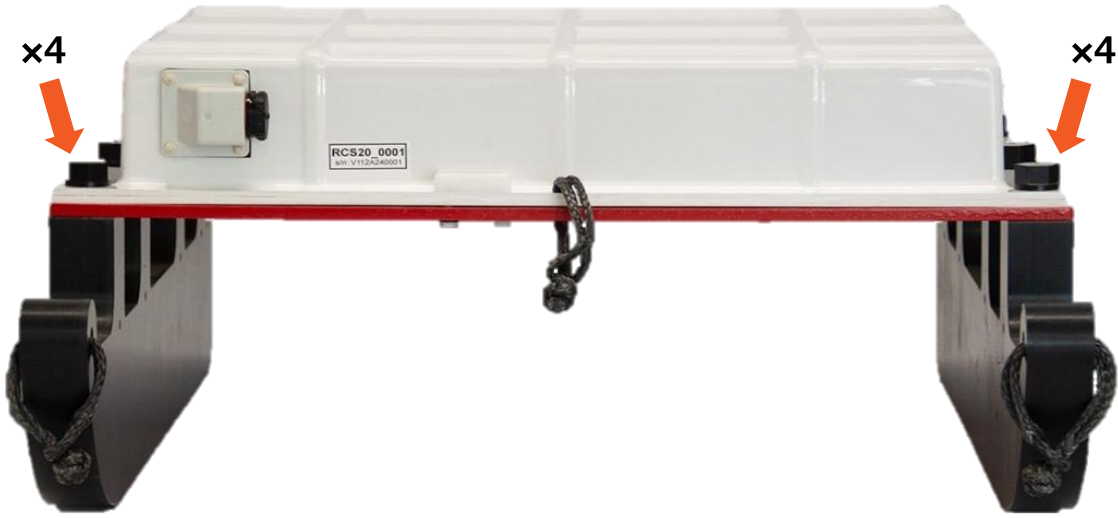
Figure 5 Receiver coil mounted on platform and secured to runners with bolts
