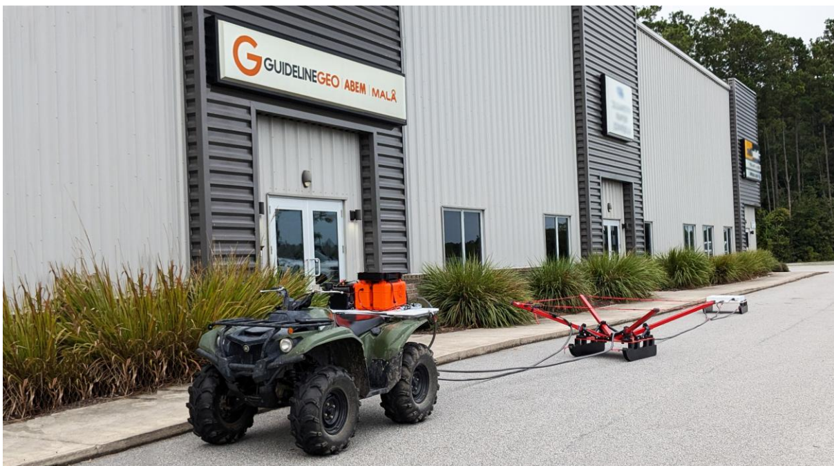
Figure 1. The ABEM GroundTEM Ralli mounted on an ATV with 2 × 2 m transmitter loop and trailing receiver coil
