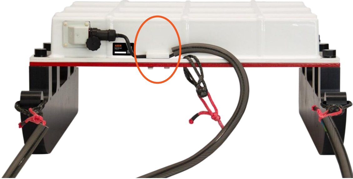
Figure 6: Connecting receiver cable to receiver platform and RCS20
