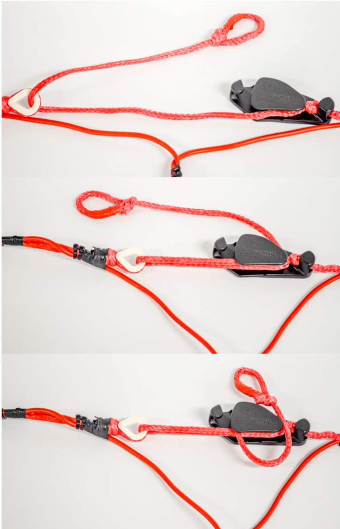
Figure 10: How to operate a cleat. Rope is loose (top), Bring rope beneath the black cleat and towards up and tighten it (middle), Lock rope by bringing it downwards to the left side of the black cleat (bottom).
