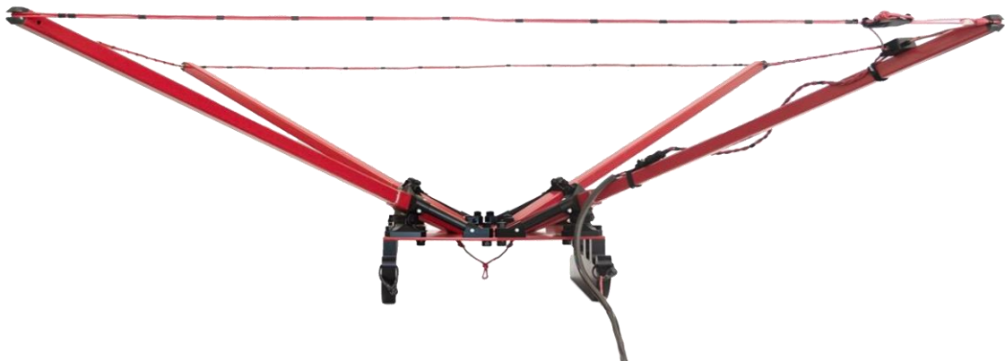
Figure 8: Example of GroundTEM Ralli system with 331 Tx coil.
