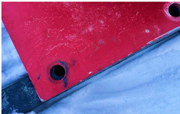
Figure 26. Example of shrank runners in extreme cold weather ( -25\text{ }^{\circ}\text{C} ).
