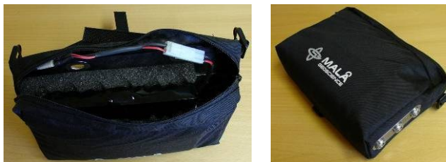
Internal of the battery pack (left) and the connectors on the outside (right)
