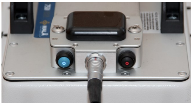
Antenna with activated Wi-Fi (blue LED)
