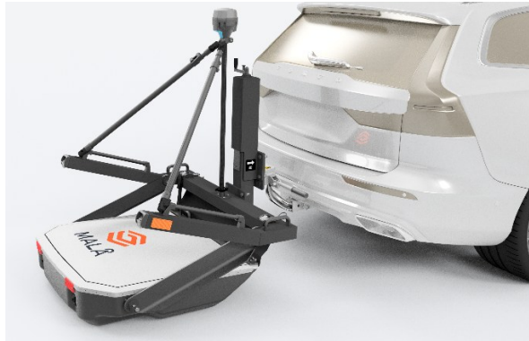
Car mount in measurement mode
