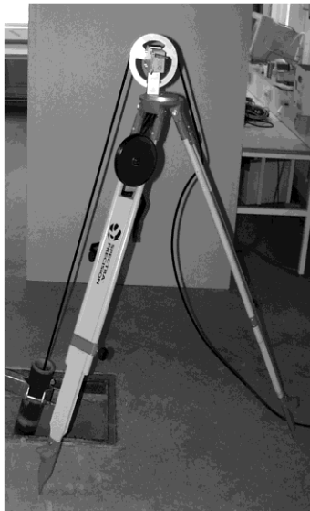
Figure 2.2. Tripod with an optical encoder.
