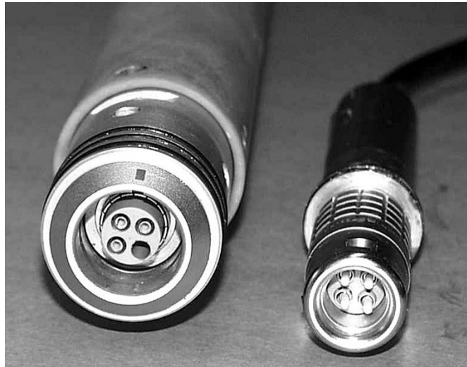
Figure 4.1. Optical connectors at probe top (Rx) and cable-head.
