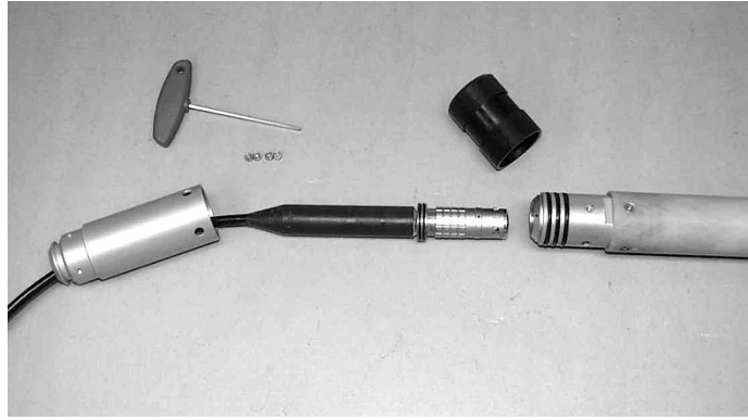
Figure 4.2. Optical cable-head including hex-tool, screws and plastic probe-top cover. The optical fiber (black) runs through the aluminum sleeve and ends with the molded optical connector. (The borehole probe top is seen to the right).
