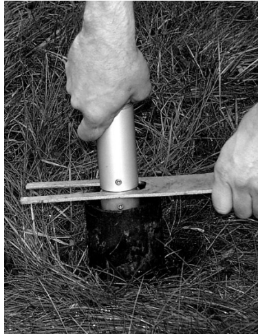
Figure 4.8 Borehole locking key mounted at cable-head of Rx antenna.
