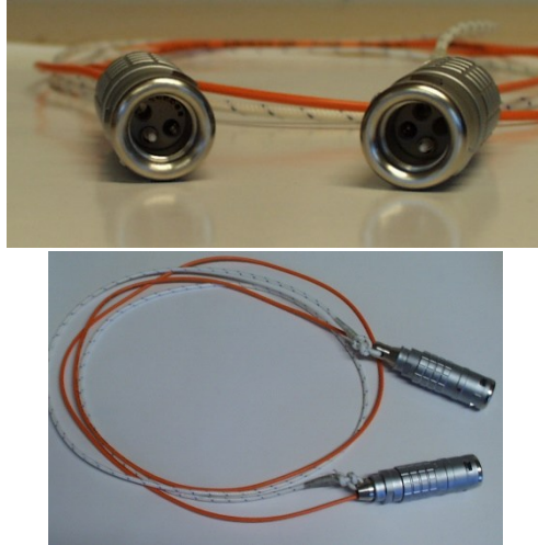
Figure 4.5. Single fiber connecting Rx to Tx.
