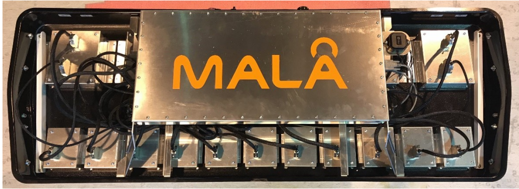
The built in GPS module can be found to the top right side of the Blockmaster
