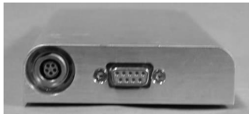
Figure 13.4 Battery pack for the RTA antennas.
