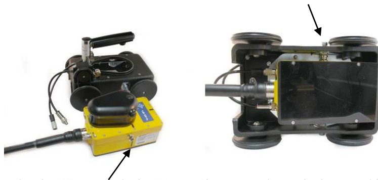
Figure 9.3 Mounting the HF antenna in the HF cart. The antenna is attached on two sides, see black arrows.
