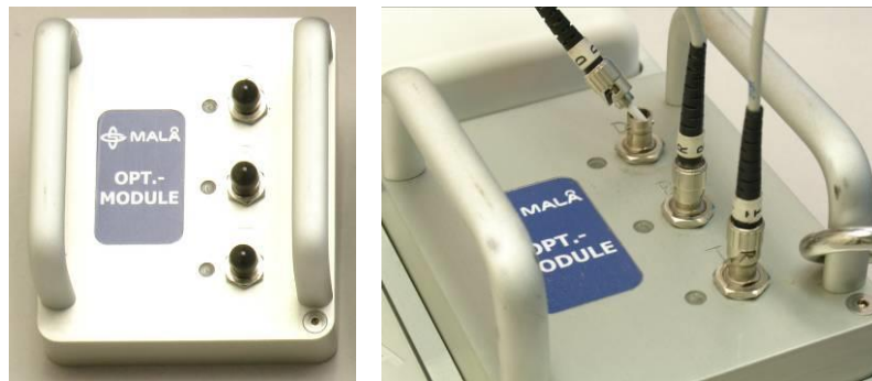
Figure 4.3 The optical module. In the picture the three different fibre optical connectors are seen, for T (Transmitter), R (Receiver) and D (Data).
