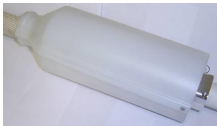
Figure 6.4 Skid plate mounted around the electronic unit.
