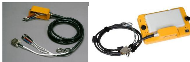
Figure 7.4 The cable hose to the shielded electronic unit (left), and the electronic unit with battery and mounted cable (right).
