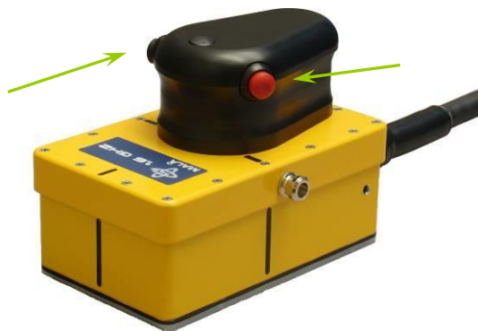
Figure 9.5 The 1.6 GHz antenna with the right (black) and left (red) hand buttons visible.
