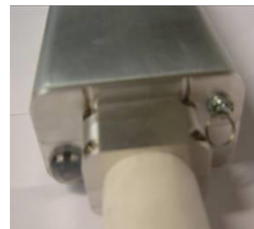
Figure 6.3 Left: Electronic unit with battery. Right: The on/off button is seen at the left side and the snap-lock for the battery on the right side.
