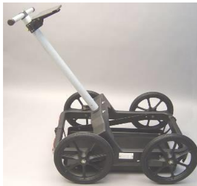
Figure 7.5 The RTC for shielded 250, 500 and 800 MHz antennas.
