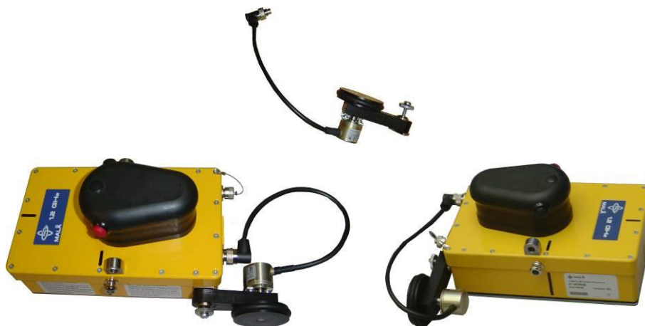
Figure 9.4 The single wheel encoder (top) and attached to a HF antenna (below) in two different directions.
