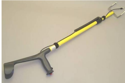
Figure 9.6 Extension pole. On the handgrip the two buttons are seen, the one on the top (red) starts a new profile.
