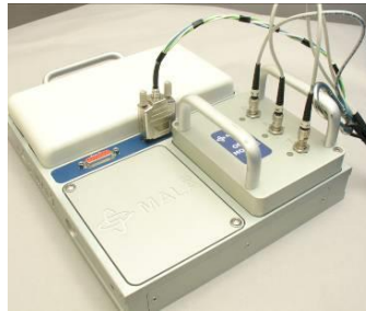
Figure 6.2 Connection to the ProEx.
