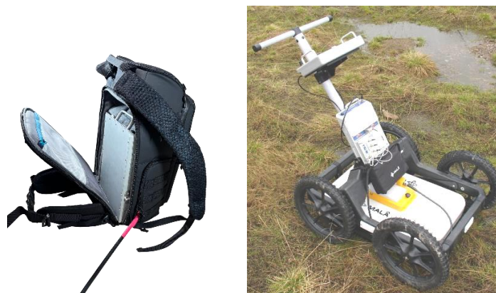
Figure 2.3 The MALÅ ProEx Control unit mounted in the MALÅ Backpack and on the RTC.
