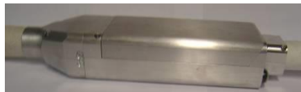
Figure 6.3 Left: Electronic unit with battery. Right: The on/off button is seen at the left side and the snap-lock for the battery on the right side.
