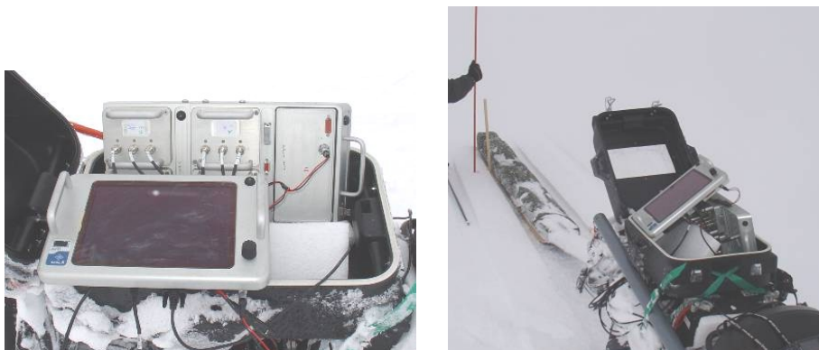
Figure 10.4 The ProEx unit installed on a snowmobile, using one expansion unit and 4 different antennas.
