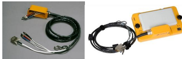
Figure 7.4 The cable hose to the shielded electronic unit (left), and the electronic unit with battery and mounted cable (right).
