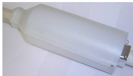
Figure 6.4 Skid plate mounted around the electronic unit.
