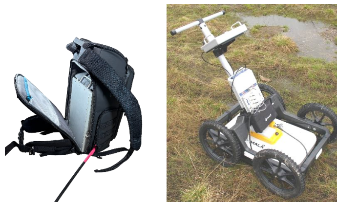
Figure 2.3 The MALÅ ProEx Control unit mounted in the MALÅ Backpack and on the RTC.
