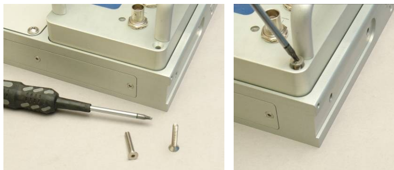
Figure 4.2. Mounting the antenna module on the ProEx main unit.
