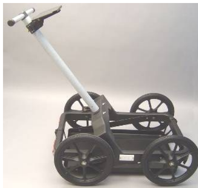
Figure 7.5 The RTC for shielded 250, 500 and 800 MHz antennas.
