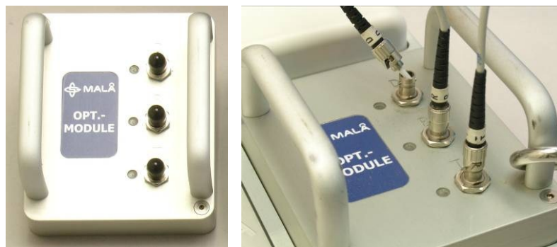
Figure 4.3 The optical module. In the picture the three different fibre optical connectors are seen, for T (Transmitter), R (Receiver) and D (Data).
