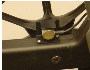
Figure 7.6 The pulse encoder on the back wheel. The screw below is for the wheel axles.
