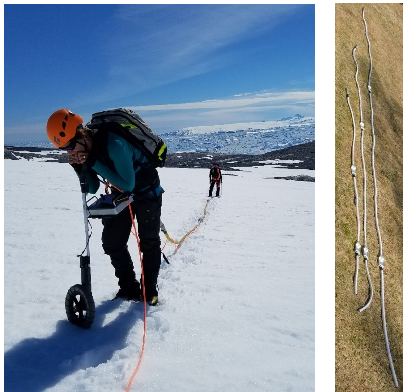
Figure 6.1 The RT antenna in field (left). The three different antenna frequencies; 100, 50 and 30MHz (right).
