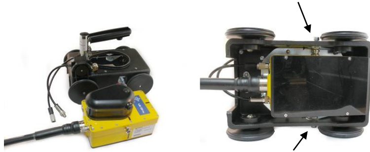
Figure 9.3 Mounting the HF antenna in the HF cart. The antenna is attached on two sides, see black arrows.
