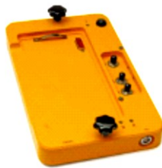
Figure 7.3 Shielded antenna electronic unit without the optical fibre cable. The connector for the external battery is seen at the front, right-hand side.
