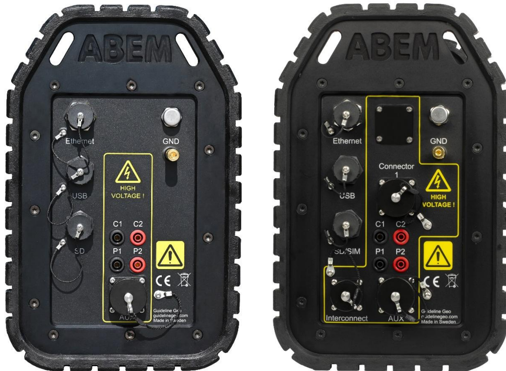
Figure 3 The connector panels of the Terrameter VES (left) and VES MAX
