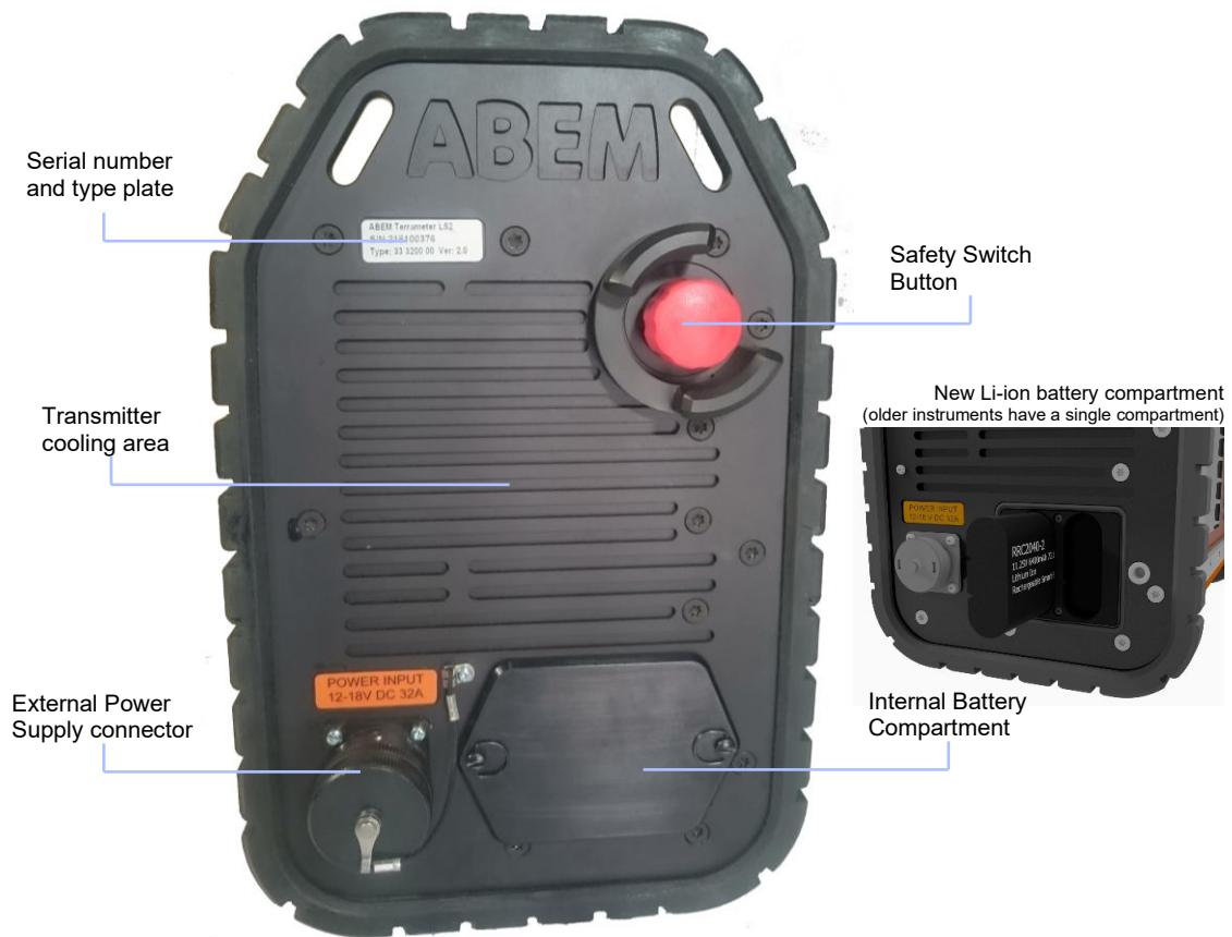
Figure 4 The power panel of a Terrameter VES / VES MAX
