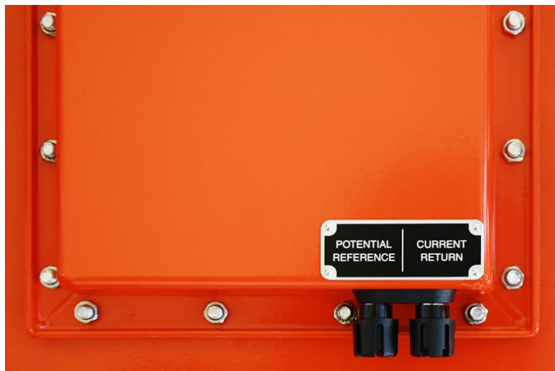
Figure 75 Connectors on the reverse of the backpacking frame
