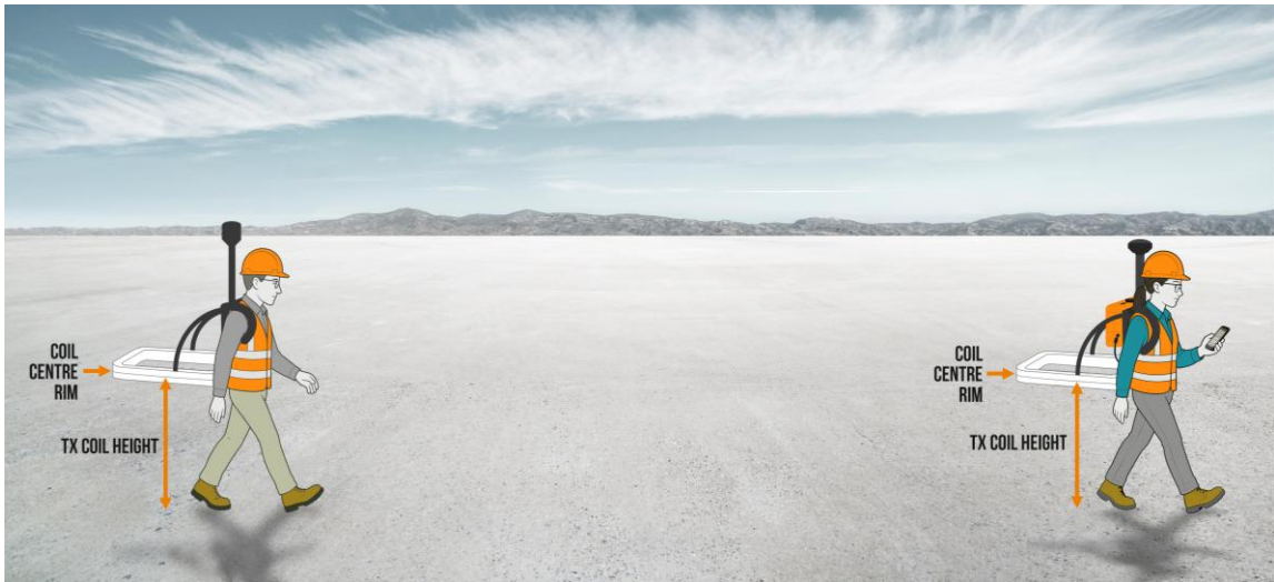
Figure 24: Depiction of proper coil height measurement
