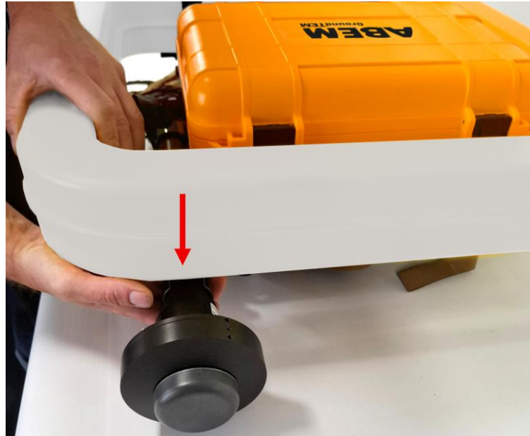
Figure 22: How to secure the Tx coil to the pole on the transmitter backpack
