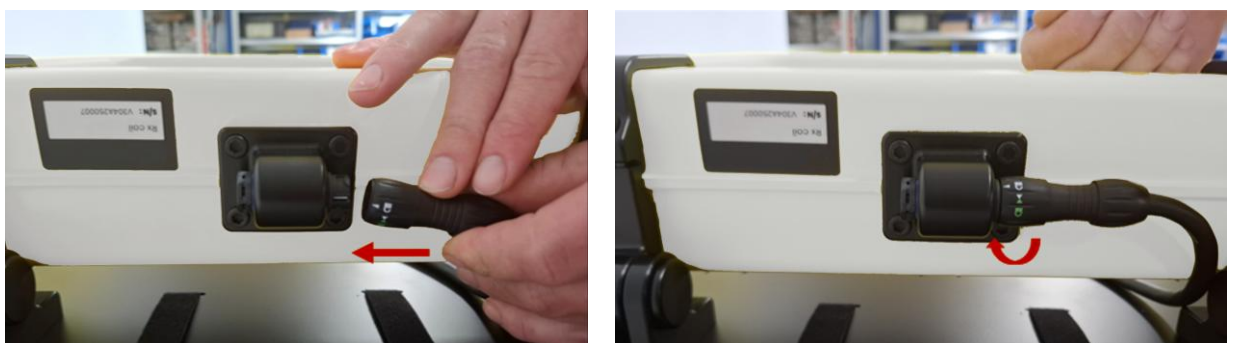
Figure 16: How to connect the Rx unit cable to the connector on the Rx coil.
