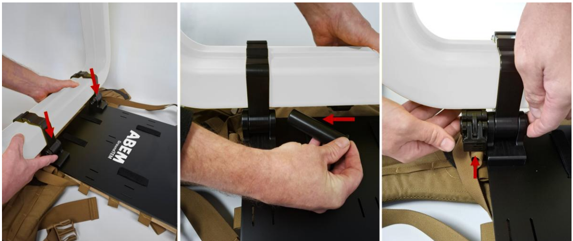
Figure 12: How to secure the Rx coil to the receiver backpack
