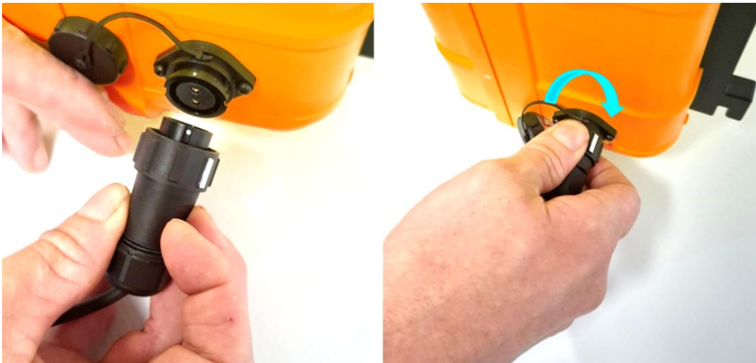
Figure 19: How to plug in the connector to the Tx unit.
