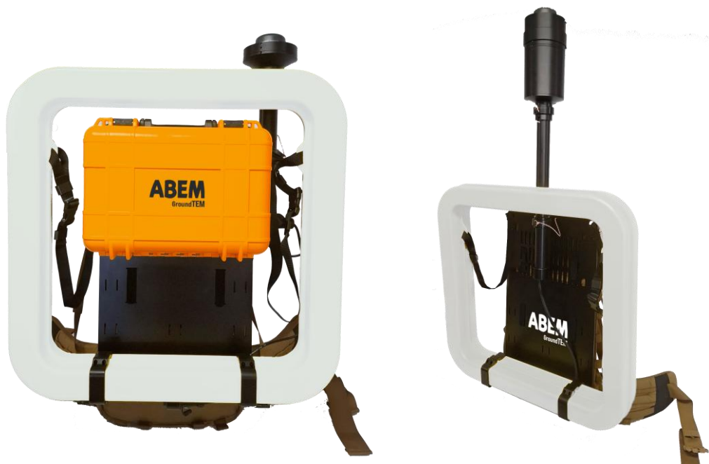
Figure 3: Assembled transmitter coil backpack (left) & receiver coil backpack (right)
