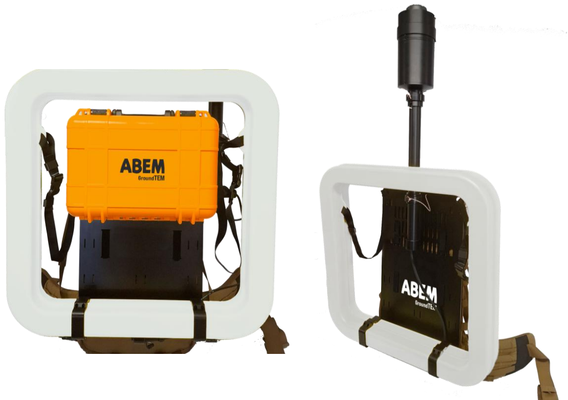
Figure 28: Assembled transmitter and receiver backpacks in locked position for comfortable transportation.
