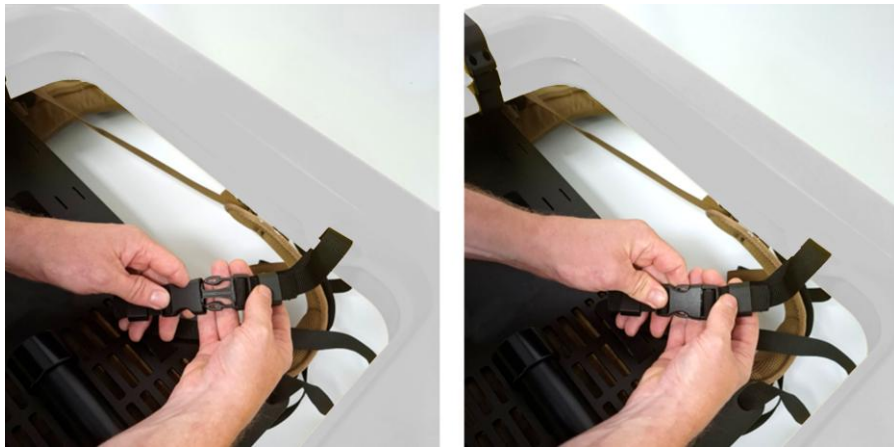
Figure 14: How to secure the straps of the Rx coil to the straps of the backpack.
